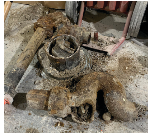
Collapsed and plugged pipes in floor drain.
